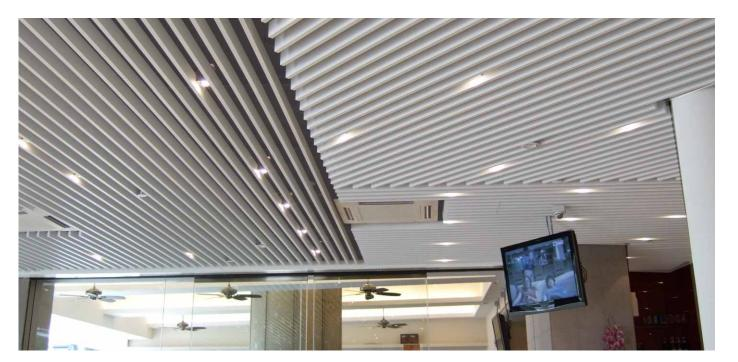
Metal Craft Linear or strip ceilings provide an aeisthetic linear finish to any interior. Available in a variety of profiles and modules, including 84R, 84C, 184C, 150F, 200F, 75C and 150C. The panels are available in coil steel and aluminum substrates. Perforated profiles are available 2.5mm and 1.7mm perforation for acoustic applications.
